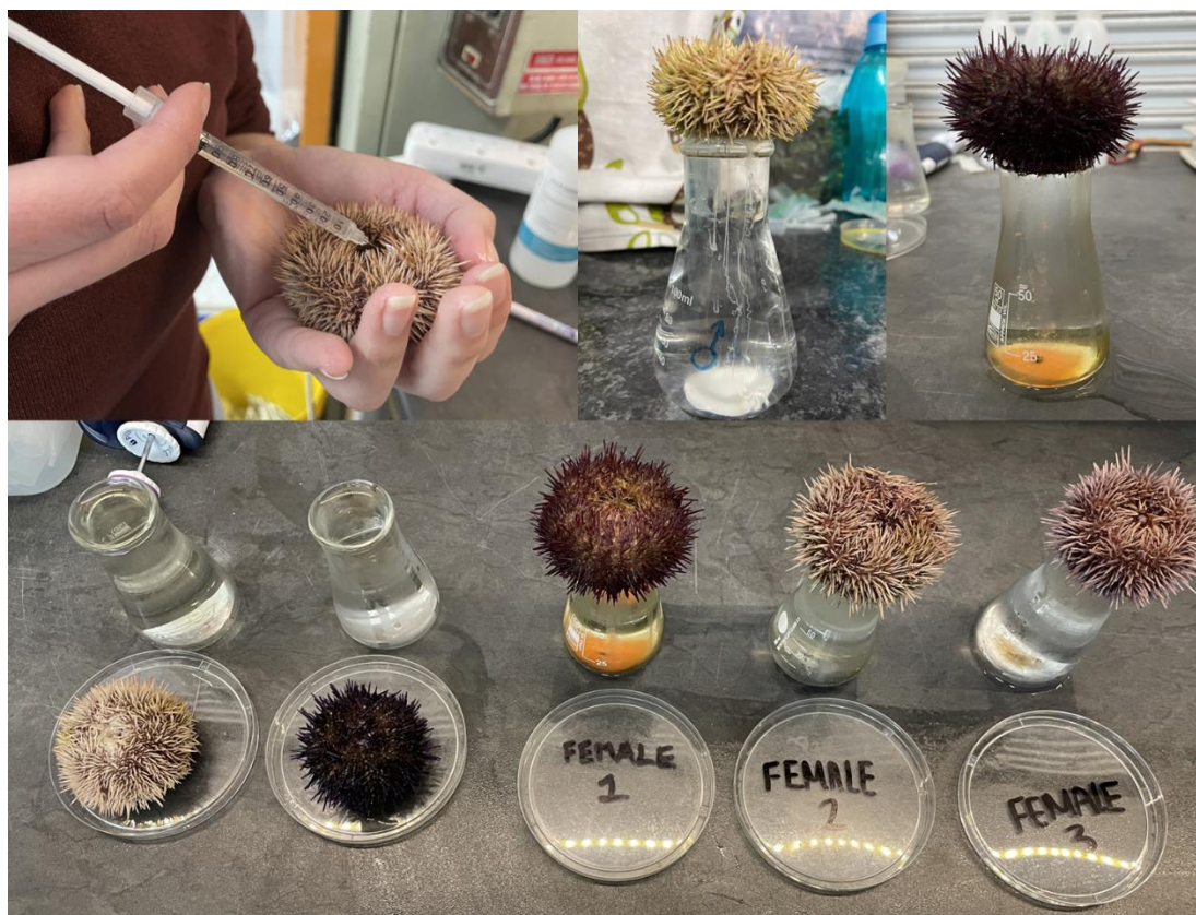
Figure 2-6. The spawning phase of seawater toxicity testing at the laboratory using the Cape Sea Urchin Parechinus angulosus .
