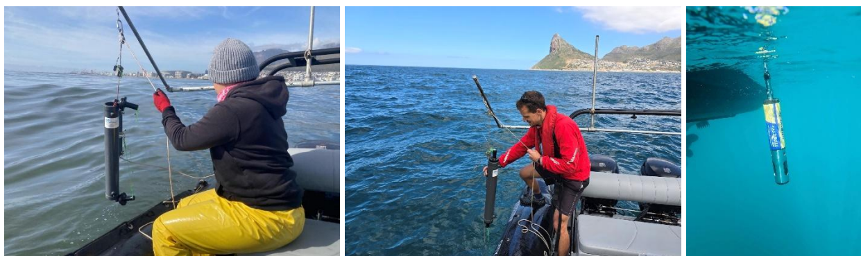
Figure 2-5. Sampling using a Niskin sampler at Green Point (left) and Hout Bay (centre), with probes (right) lowered to the appropriate depths for in situ measurements
