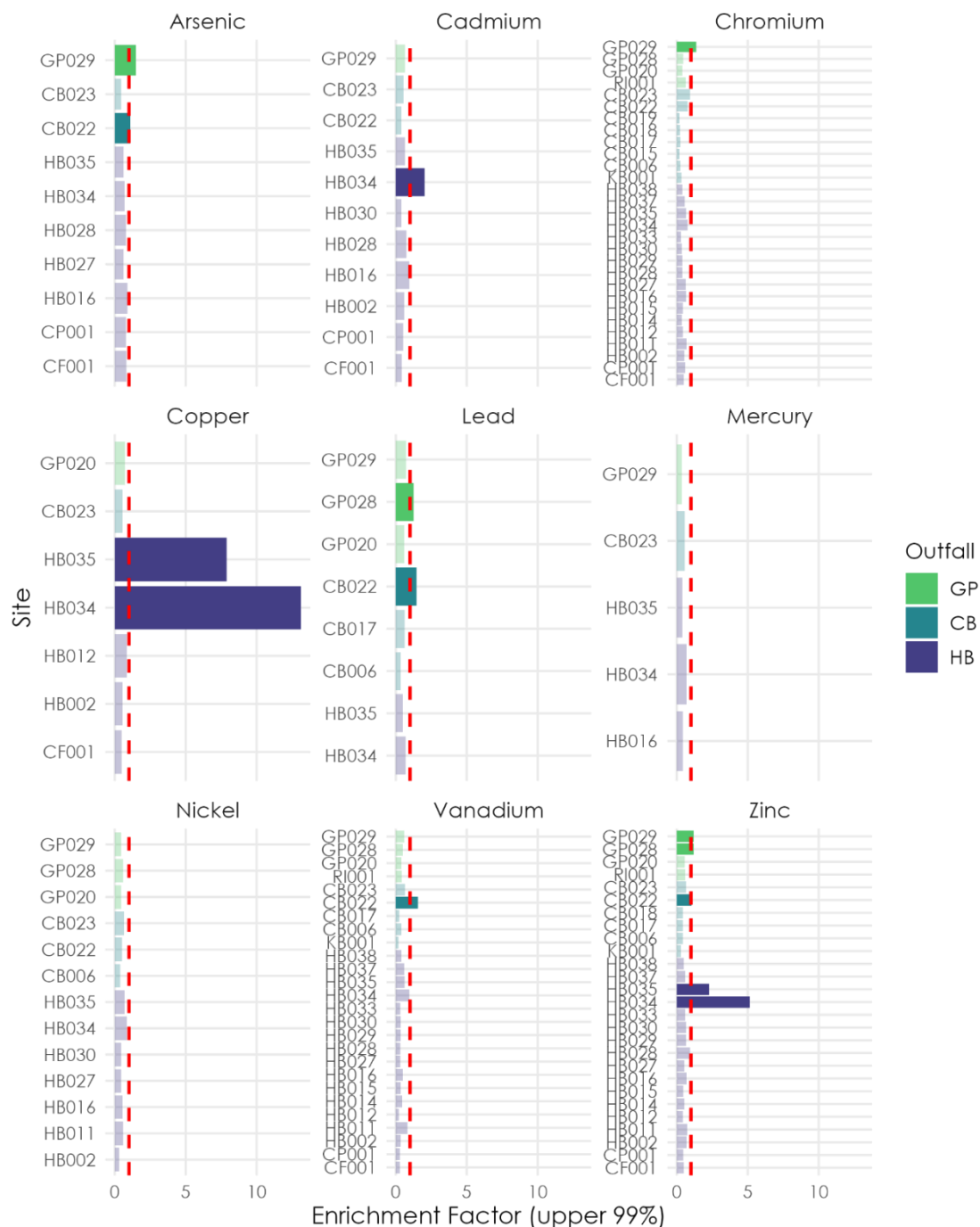
Figure 4-5. Sediment metal enrichment factors from Green Point, Hout Bay and Camps Bay in 2025. Non-faded bars exceeded the 99% upper prediction interval of the CSIR baseline model (red dashed line), signifying likely anthropogenic enrichment. Where a metal was below the laboratory lower detection limit, the site was not included on the plot.
